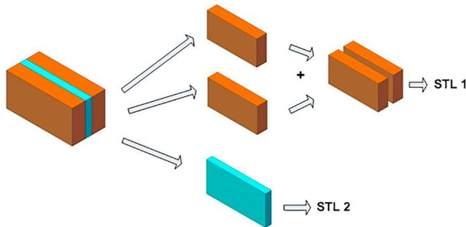
Fig. 5. Multiple STL files for multi-material components.
